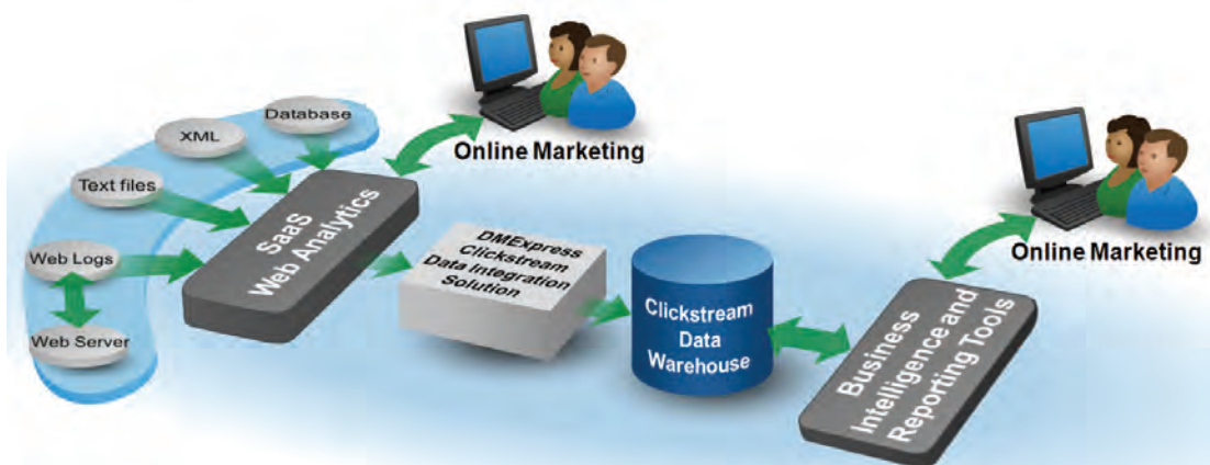
Figure 3. Typical architecture of a clickstream data warehouse implementation with DMExpress
